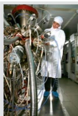
Fig. 15.1 Basic research conducted within the framework of the NCCR “Quantum Photonics” leads to the development of new products. The technique of molecular beam epitaxy (MBE) makes it possible to grow the single crystal layers of semiconductor compounds. This technique is used most notably for the manufacture of optoelectronic components such as laser diodes or quantum cascade lasers.
