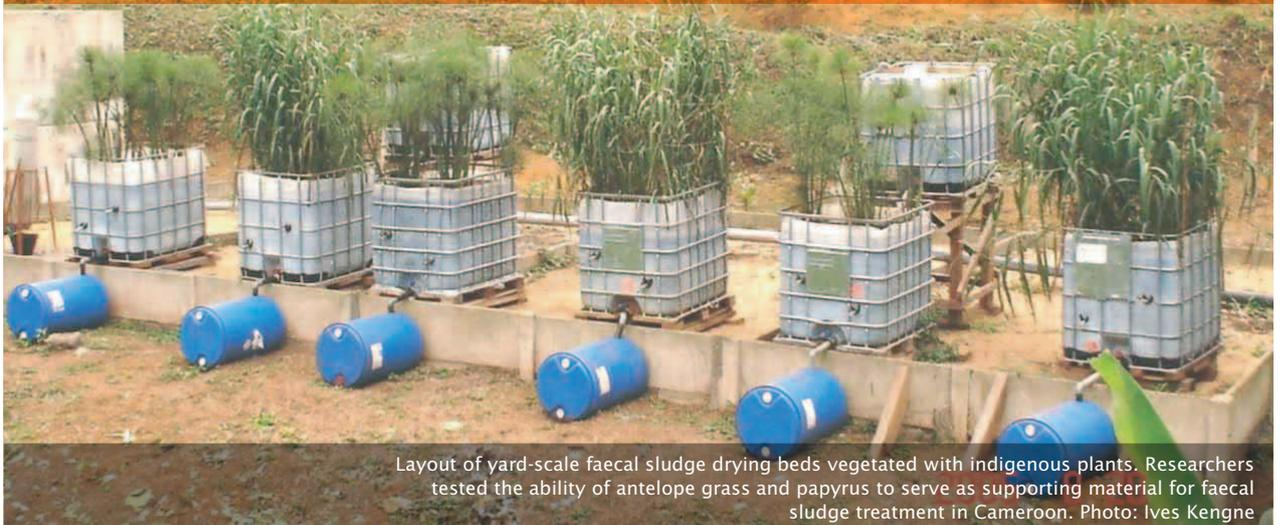
Layout of yard-scale faecal sludge drying beds vegetated with indigenous plants. Researchers tested the ability of antelope grass and papyrus to serve as supporting material for faecal sludge treatment in Cameroon. Photo: Ives Kengne
